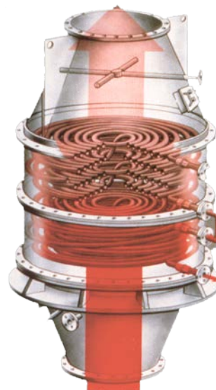
EXHAUST GAS BOILER
